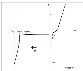
Fig. 3. V-I characteristics for a unidirectional ESD protection diode
