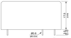
Dimensions in mm (inch) Tolerances:  $x.x \pm 0.5 (\pm 0.02)$
