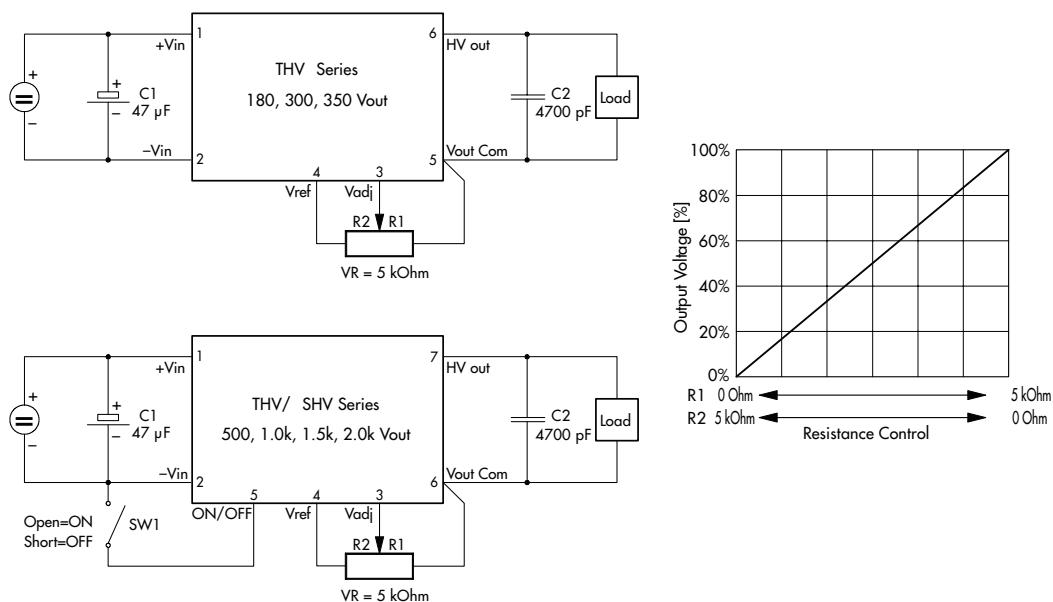
Connection for remote control voltage control
