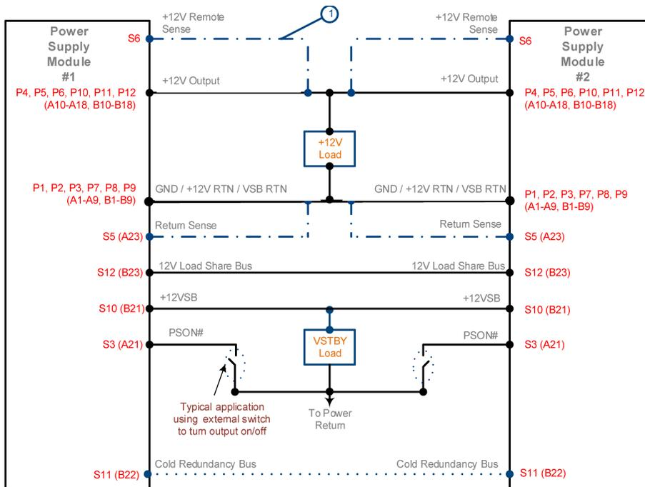
1) Dotted lines show optional remote sense connections. Optional remote sense lines can be attached to a load that is a distance away from the power supply to improve regulation at the load
