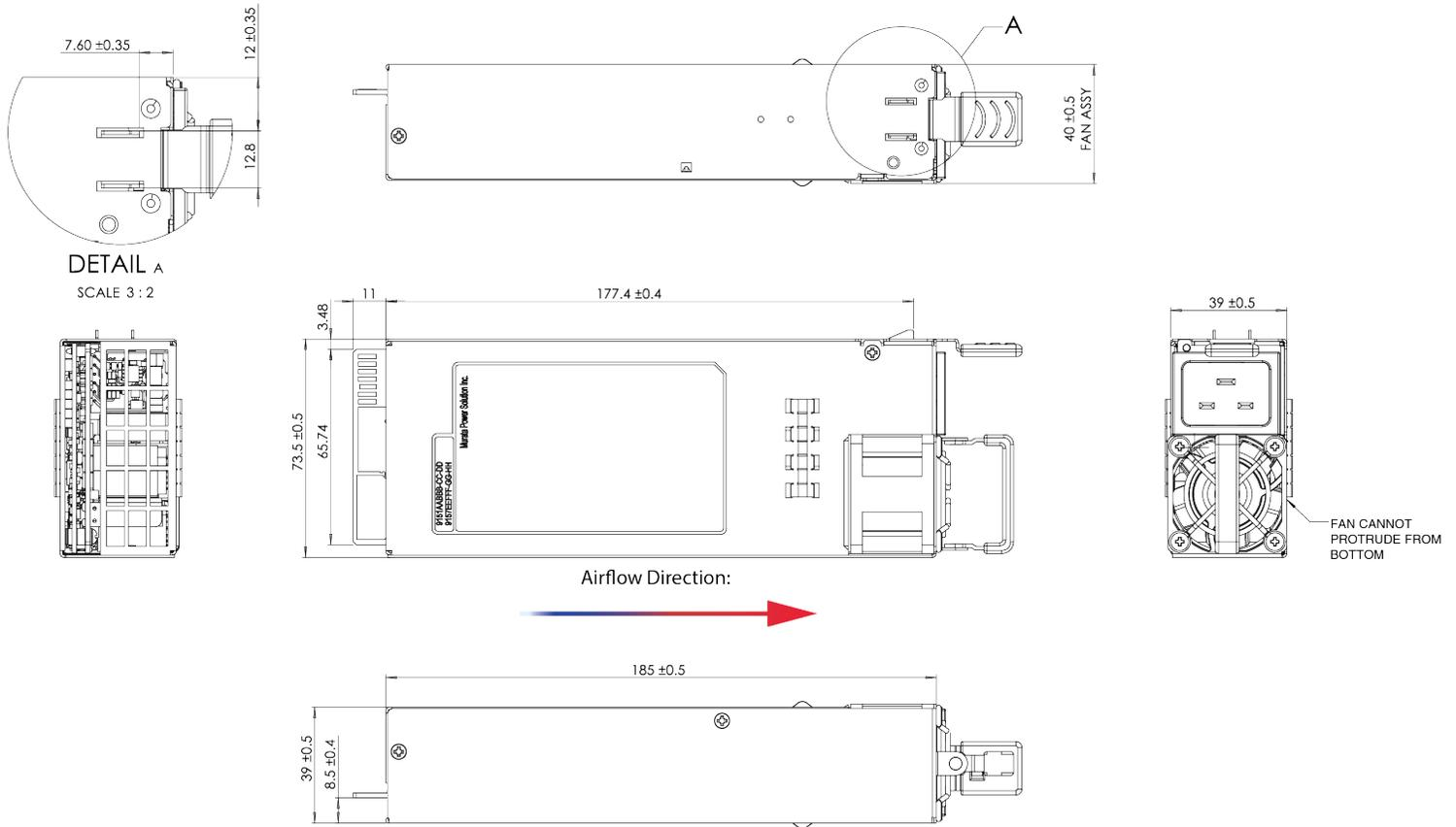
1. AC input connector: IEC 60320-C20
